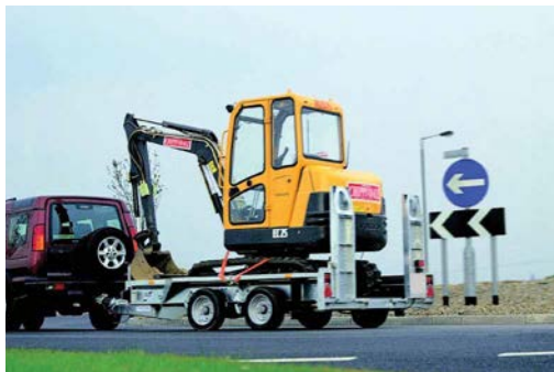
GX105 10' x 5' Plant Trailer 3500kg Gross Shown with skids. Also available with ramp
