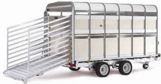
DPI20G 12'x6'6" Dual Purpose Livestock Trailer (Wheel underneath/removable container. Available with removable Low Loading Drop Sides as an optional extra). With or without Fold-up Sheep Deck.
