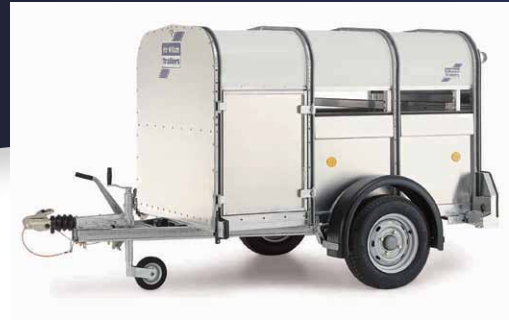
P6G 6'x4' Pig and Sheep Trailer Single Axle (Braked). Pig and Sheep Trailer is fitted standard with rear ramp, aluminum loading gates and spare wheel.
