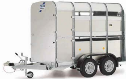
TASG 8'x5'x6'H Livestock Trailer (Available with or without Fold-up Sheep Deck) Twin Axle. Fitted standard with rear ramp, aluminum loading gates and spare wheel.
