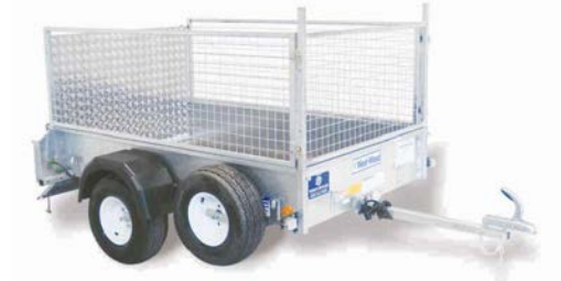
P6e 6'6" x 4' Galvanised Car Trailer with high loading ramp and mesh sides. 500kg gross capacity (On balloon flotation wheels). For on or off road use.
