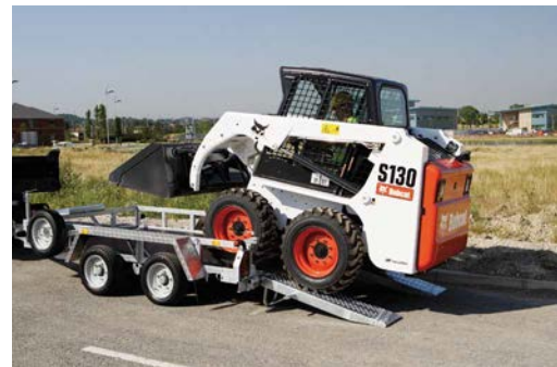
GP106 10' x 5'10" Plant Trailer 3500kg Gross Shown with open low sides and skids
