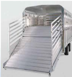
Easy Load Fold-up Hydraulic Sheep Deck System.
