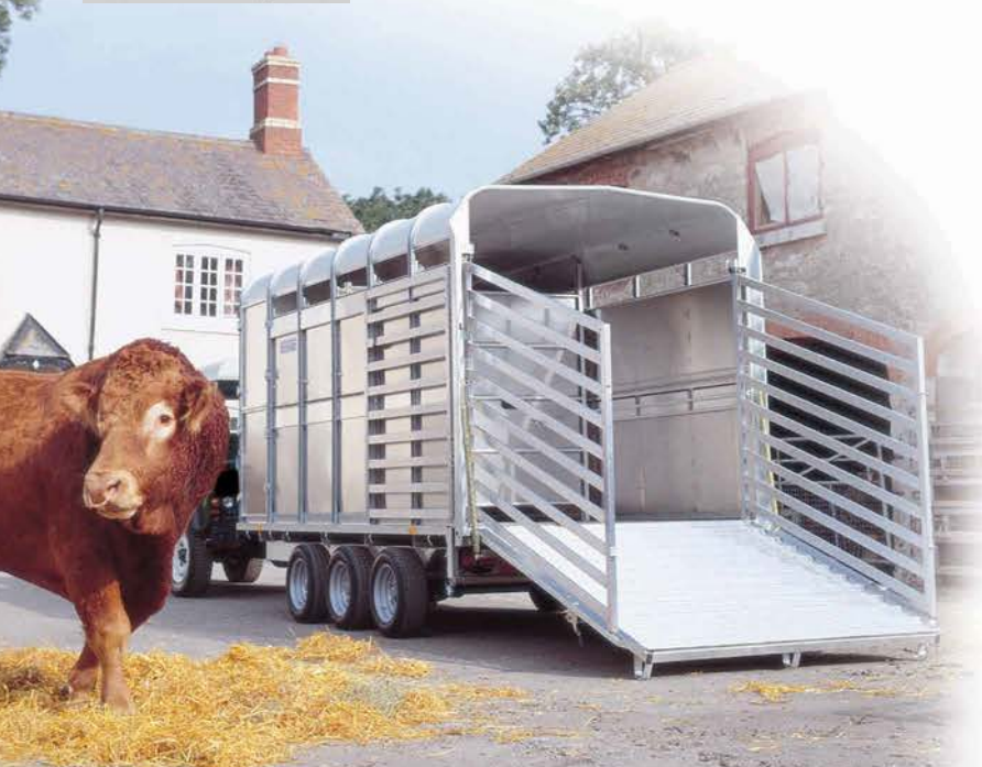
TASG 10'x5'x6'H Livestock Trailer (Available with or without Fold-up Sheep Deck). Twin Axle. 175 x 16 Landrover wheel equipment. Model available with 7' headroom for horses (see opposite).
