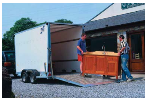
BV126G 12' x 5'10" x 7' Box Van 3500kg Gross Choice of roller shutter or ramp/door combination
