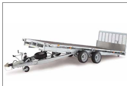
CT166G 16' x 6'6" Twin Axle Tilt Bed Shown without optional dropsides in loading position
