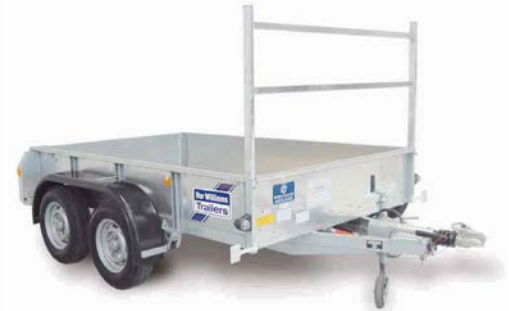
GD85G Twin Axle 8'x5' General Duty Trailer. 2700kg gross capacity. (Optional Ladder Rack as shown). Full range of accessories can be added to this trailer.
