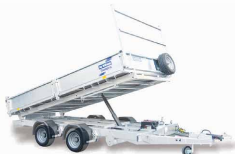
TT126G 12'x6'6" Tipping Trailer. 3500kg gross capacity. Electric model. Fitted with alloy floor and ladder rack as standard on this model.
