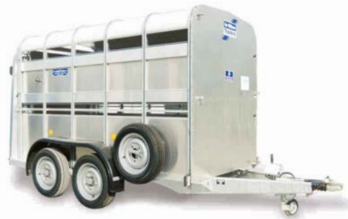
TASG 10'x5'x6'H Livestock Trailer (Available with or without Fold-up Sheep Deck). Twin Axle. 175 x 16 Landrover wheel equipment. Model available with 7' headroom for horses (see opposite).
