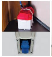
Electric Power Source There is the option for either a 12v or 230v power source supply to your trailer. The 12v source is an on-board supply. The 230v option is a socket for connecting to an external main source.
