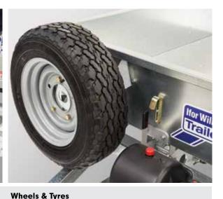
The trailer is fitted with the rugged 185/70R13C tyres, with a spare wheel fitted as standard.
