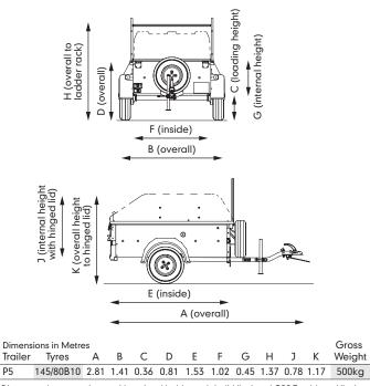
Diagrams above are shown with optional ladder rack (solid line) and GRP Top (dotted line) See inside back cover for unladen weight.
