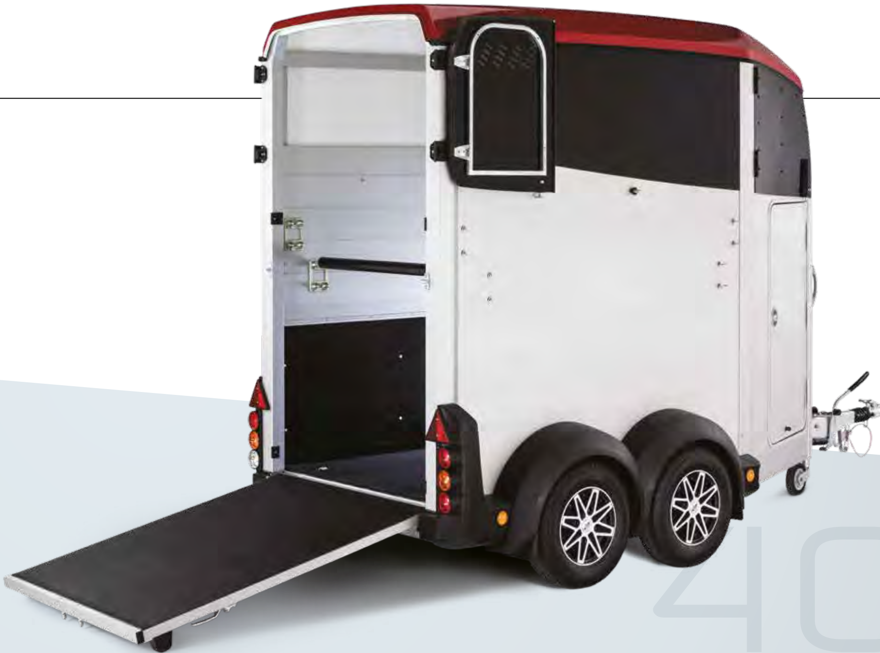
HBX-403 In red, with left hand front ramp and 8-spoke diamond cut alloy wheels
