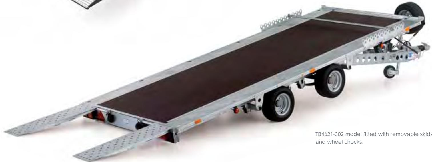
TB4621-302 model fitted with removable skids and wheel chocks.
